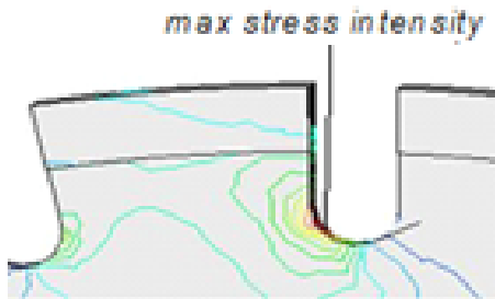
Fig. 2. Isolines of stress intensity from cutting forces
