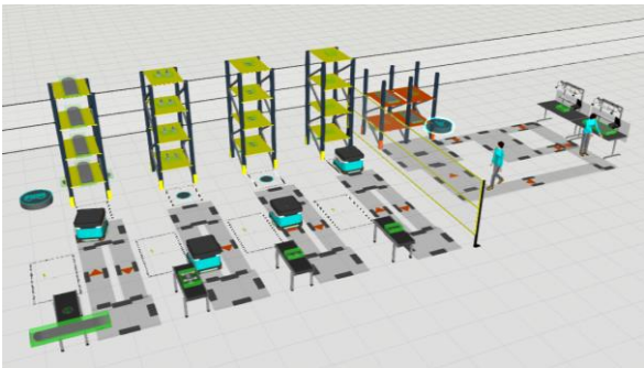
Fig. 9. A model of moving parts using humans and robots to assemble a skateboard.
